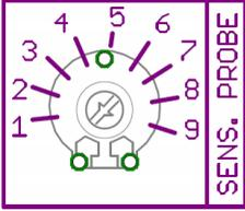
The trimmer “SENS. PROBE” can be used to adjust sensitivity of the sensors to adapt them to conductivity of the liquid. This value should therefore be increased in the case of liquids with low conductivity.
