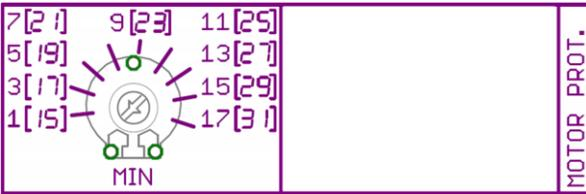
The “MIN” trimmer enables adjustment of the minimum motor current for protection against the risk of dry running, for added protection or when minimum level floats or sensors are not required.
