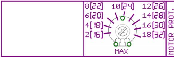
The "MAX" trimmer enables adjustment of the maximum motor current, over which the system protection trips due to current overload.
