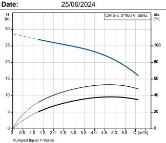
Liquid temperature during operation = 20 °C
